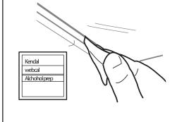
Apply primer at installation points. Wait - 30 secs. The purpose is to increase adhesive efficiency between surface and tape.
