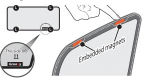
Apply primer ONLY if surface has been treated or polished Place the L-Clips at the magnet locations of the sunshade. Note: Do not remove protective layer on adhesive tape Embedded magnets
