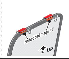
Place sunshade with the L-clips attached to the panel of the sunroof to find the position for the sunshade and L-clips.
